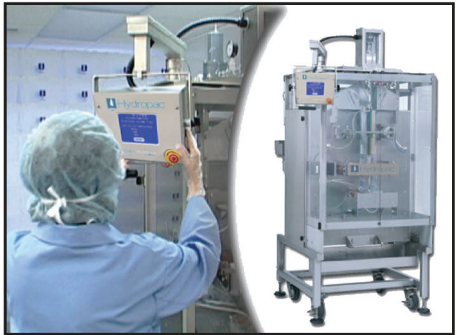
Figure 1. The Hydropac™ AWS-5000 Pouch Machine automatically forms, fills, and seals pouches using a continuous roll of special plastic film stock. A touch screen panel located on an articulating arm activates all control functions.
